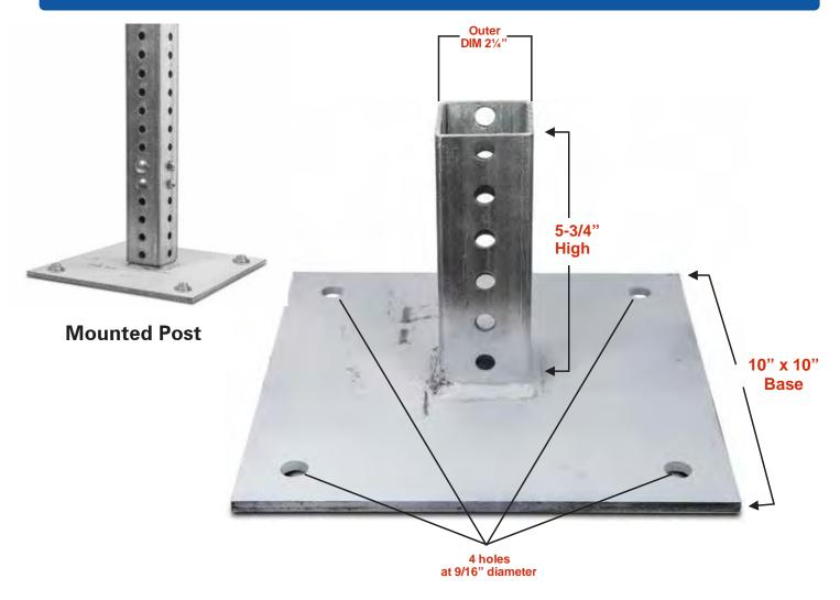
The square post surface mount base is a great choice when you need to install a sign post in concrete or asphalt surfaces and don't want to cut through them to install the post. Made of galvanized steel for durability. It has four 9/16" mounting holes in each corner of the base plate for anchoring the base to the ground.
